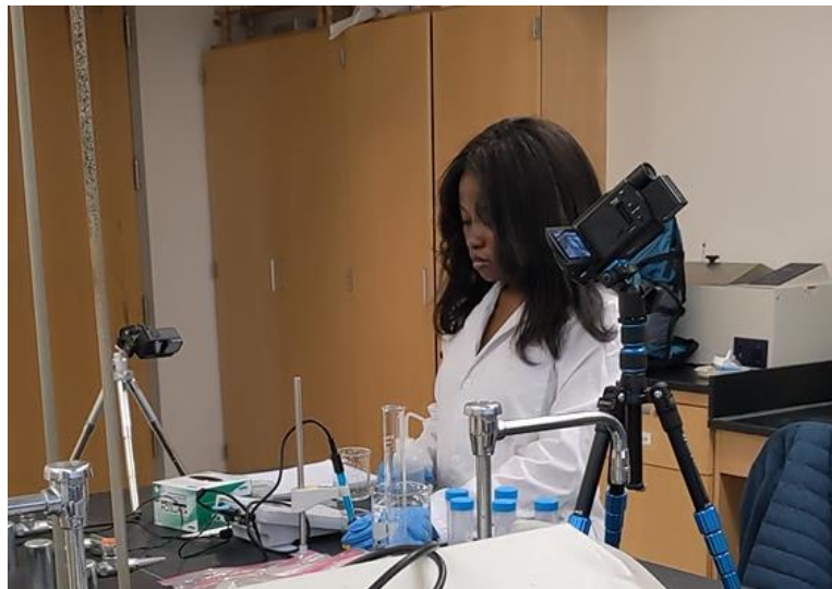
One of the interns measuring the soil PH using a digital pH meter. It was also filmed to create a short educational video.
